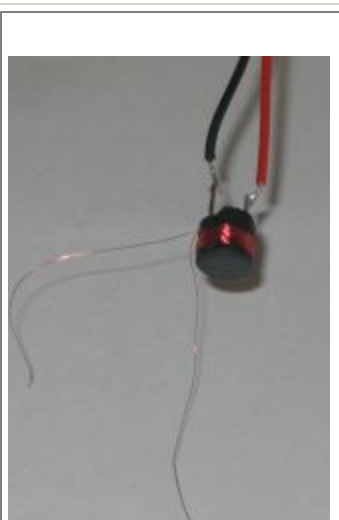
The 10mH choke with 150 turns for the secondary
