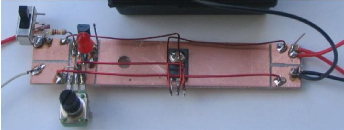
This power supply can be built in less than an hour on a piece of copper-laminate. The board acts as a heat-sink and the other components can be mounted as shown in the photo, by cutting strips to suit their placement.
